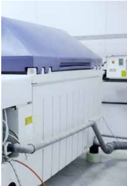
Corrosion Test - Salt-acetic fog chamber
